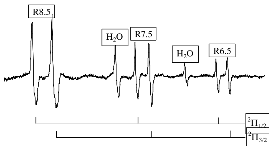
Fig. 2 Part of the absorption spectrum of NO and \text{H}_2\text{O} between 1907 \text{cm}^{-1} (left) and 1898 \text{cm}^{-1} (right).
